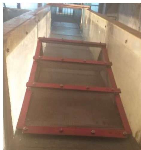
Fig. 4. Model of the elastic debris flow-regulating barrage in the hydraulic duct
