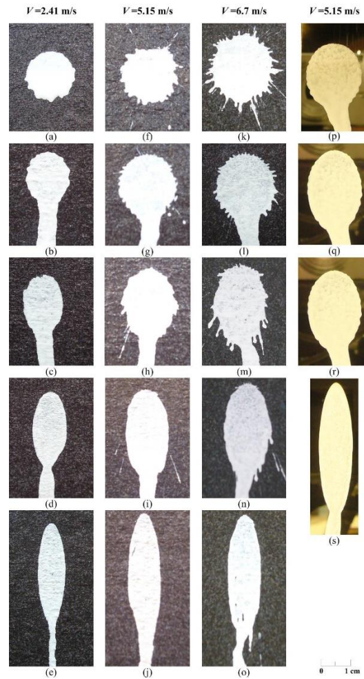
Fig. 8. Splatters left on different surfaces under different impact conditions. (a)~(e) represent on brick surface, V = 2.41 m/s, \theta = 75^\circ, 60^\circ, 45^\circ, 30^\circ, 15^\circ . (f)~(j) represent on brick surface, V = 5.15 m/s, \theta = 75^\circ, 60^\circ, 45^\circ, 30^\circ, 15^\circ . (k)~(o) represent on brick surface, V = 6.70 m/s, \theta = 75^\circ, 60^\circ, 45^\circ, 30^\circ, 15^\circ . (p)~(s) represent on mirror surface, V = 5.15 m/s, \theta = 60^\circ, 45^\circ, 30^\circ, 15^\circ
